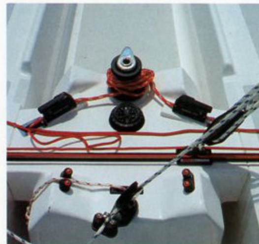
THE RUNNING BACKSTAYS, COMPASS, MAIN-SHEET, PERMANENT BACKSTAY AND TRAVELLER CONTROL WITHIN REACH FOR THE HELMSMAN. ALL LOCATED IN THE CENTRE OF THE COCKPIT.
