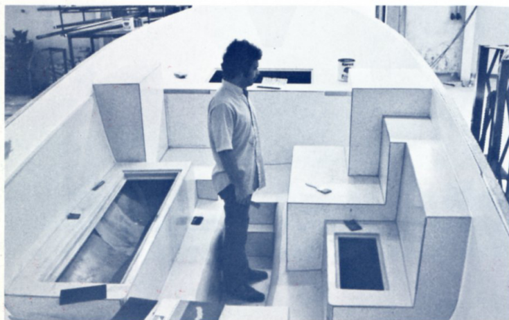
Photo shows workman standing in keel recess during process of fairing plug for production of molded, one-piece inner liner. Note step up to forward compartment.
