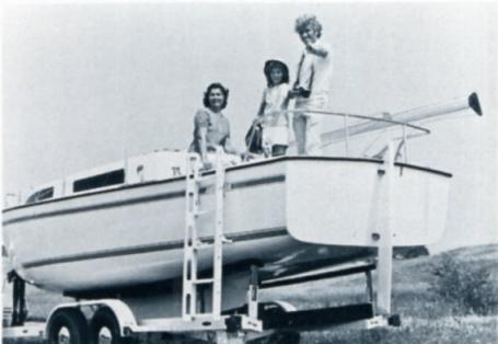
Her broad stern section gives her a buoyancy aft which makes her float off her trailer easily and early without having to back the towing car up to the hubs in water. Recovery is equally
