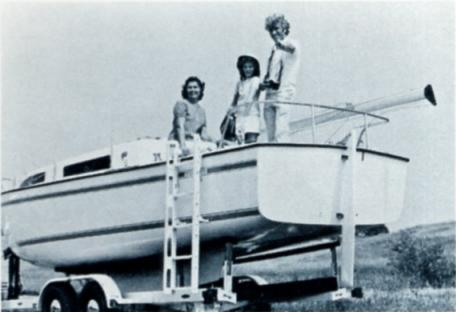
Her broad stern section gives her a buoyancy aft which makes her float off her trailer easily and early without having to back the towing car up to the hubs in water. Recovery is equally
