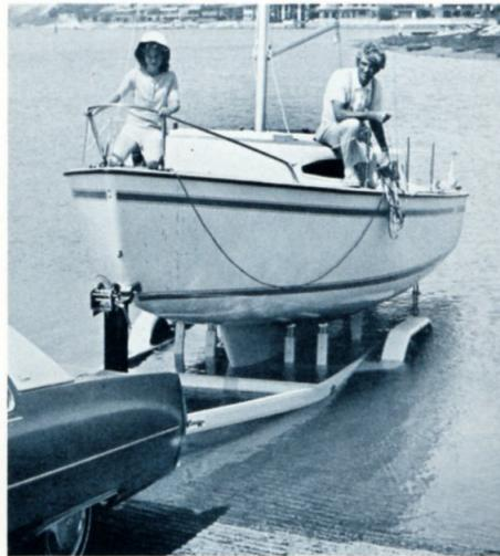
There is no "rudder struggle" involved in launching this boat. No straining to set the rudder in place *after* launching and with the boat afloat. Bouyancy does it again! You simply set the rudder pintles into their fittings *before* launching and back right into the water. No danger of it bumping or hanging up on the bottom with resultant damage. And leave it on the transom when bringing the boat ashore. In fact—just leave it there period. Even for cross-country trailering.
