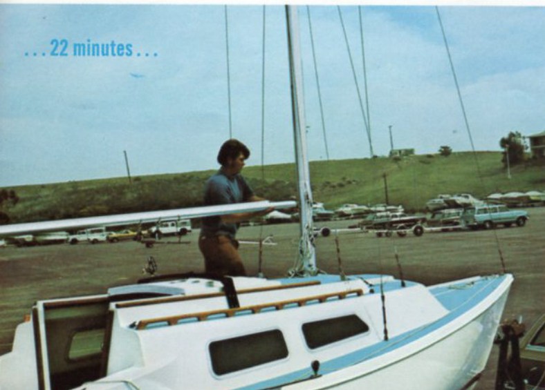
Fit boom to mast
