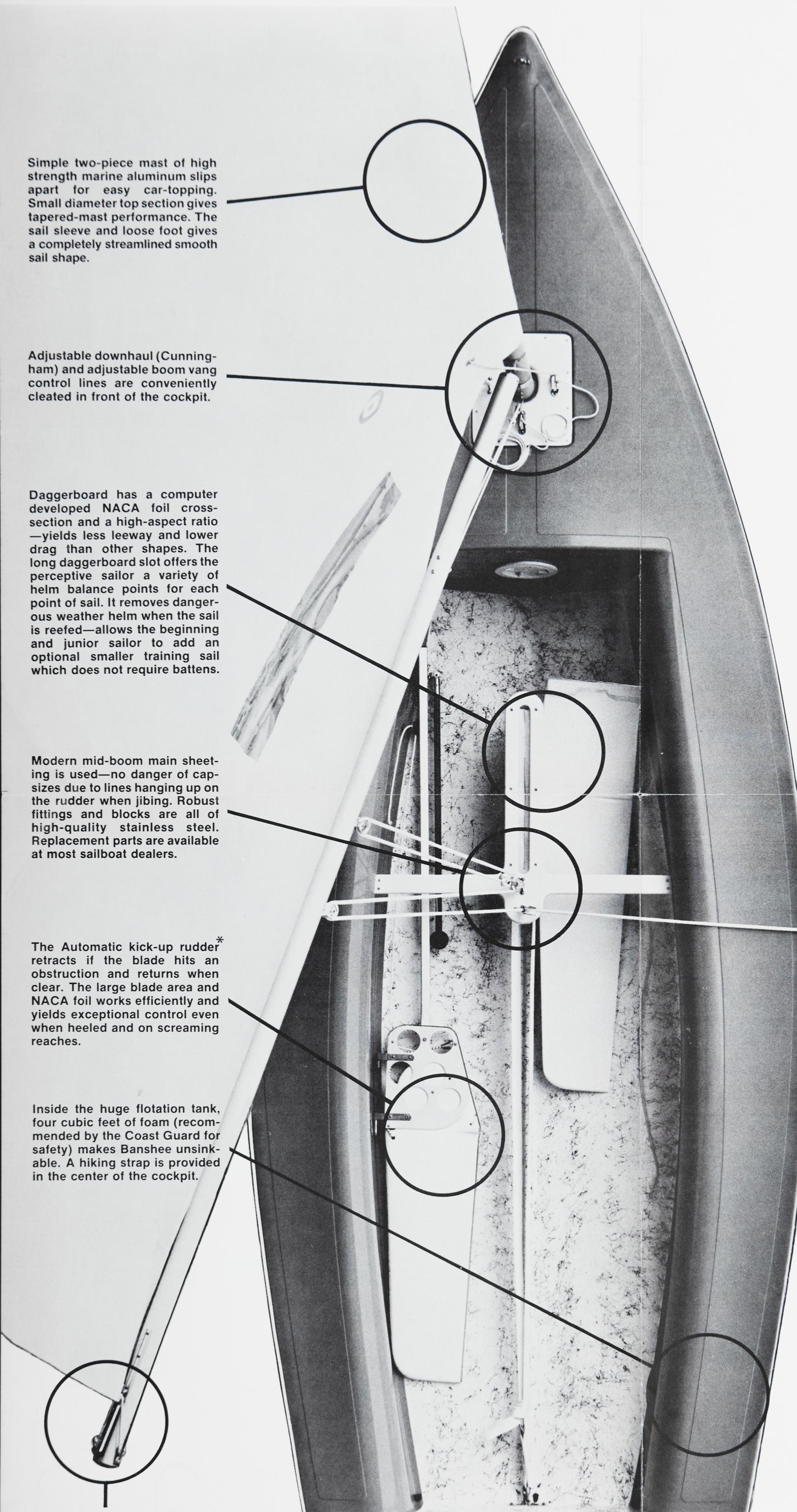
Simple two-piece mast of high strength marine aluminum slips apart for easy car-topping. Small diameter top section gives tapered-mast performance. The sail sleeve and loose foot gives a completely streamlined smooth sail shape.
