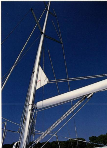
► The double spreader, furling mast has discontinuous rigging and forward lower shrouds. The furling mainsail is controlled by an inhaul and an outhaul line led aft to the maneuvering winch. All lines running aft from the mast to the cockpit are covered by a deck cowling.
