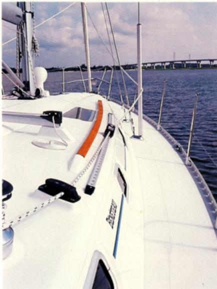
▲ Genoa tracks and turning blocks are placed on the cabin top as is the mainsheet traveller. This positioning improves the sheeting angle of the genoa and enhances upwind performance. It also clears the side decks making them safer to use.
