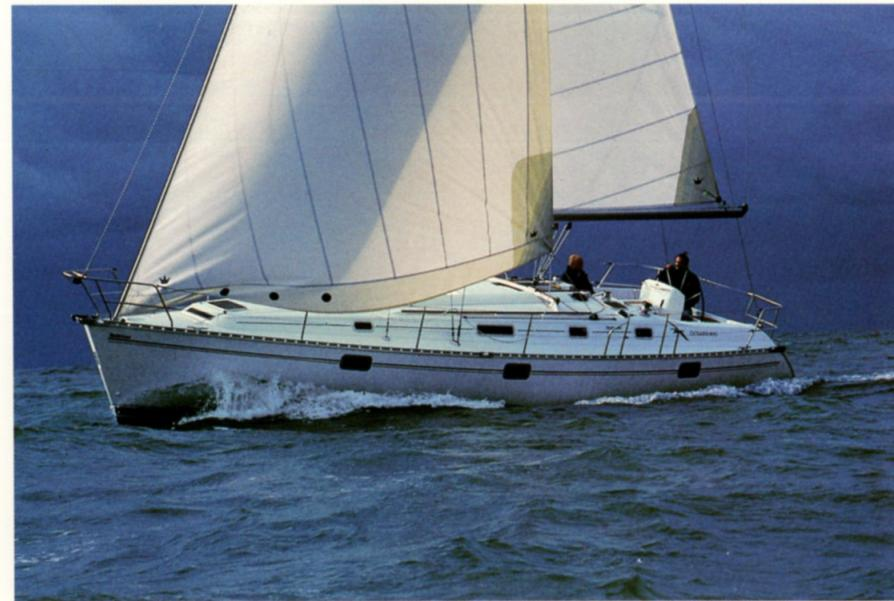
Her fin keel with bulb has a low center of gravity which allows her to sail efficiently on all points of sail while providing excellent stability. The large diameter, leather sheathed wheel, coupled to a counter-balanced rudder, provides precise and easy steerage under sail or when maneuvering under power in tight quarters.
