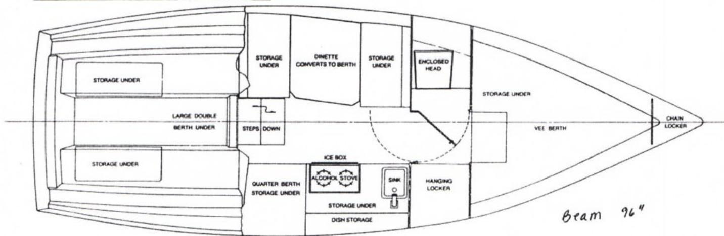
The Buccaneer 240 is designed to provide maximum cruising accommodations in a trailerable sailing yacht. Inside cabin has 6-foot headroom with a flat floor, V-berths in a privacy cabin forward, a dinette that seats four and converts to a double berth, a quarter berth,
