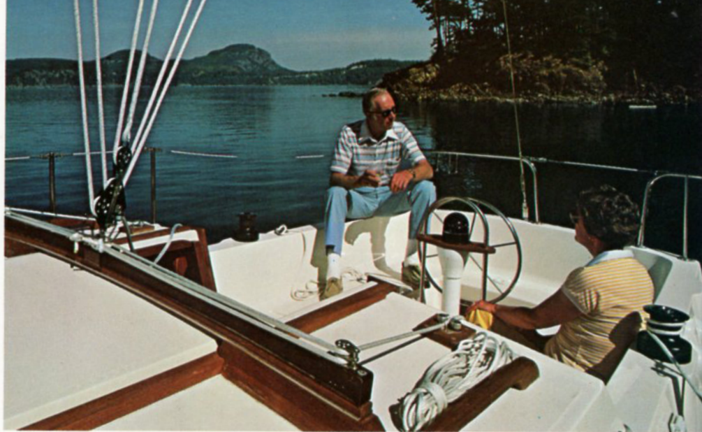
Mainsheet traveler is standard on most models; on the 305, you get pedestal steerer.
