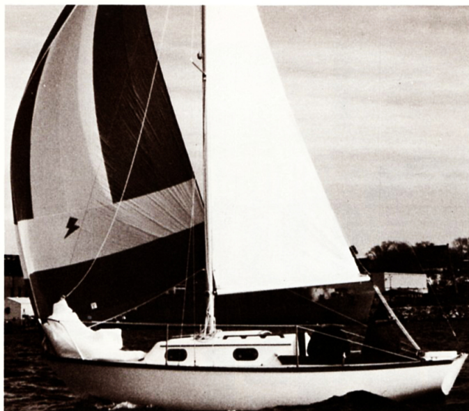
CAPE DORY 22 22D L.O.A. 22' 4" L.W.L. 16' 3" Beam 7' 4" Draft 3' 0" Displacement 3,200 lbs. Ballast 1,400 lbs. Sail Area 240 sq. ft. Designer Carl Alberg
