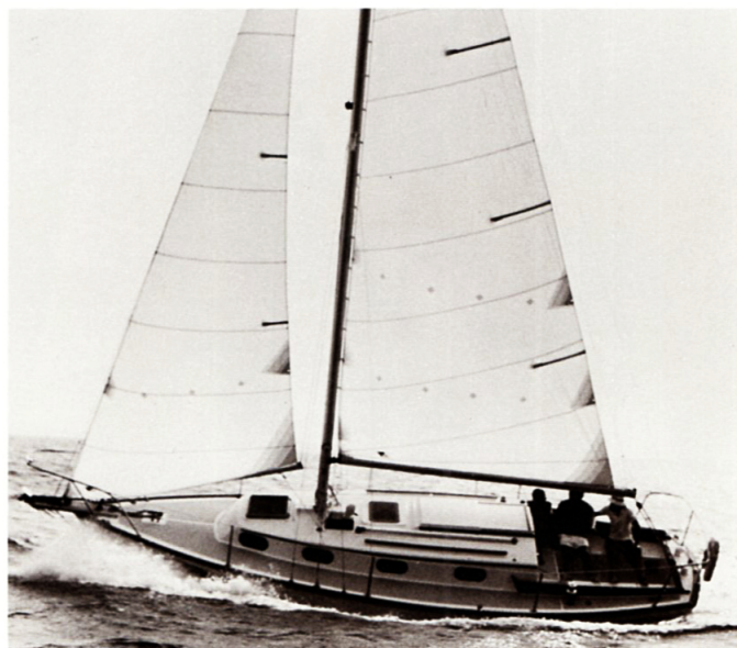
CAPE DORY 28 L.O.D. 28' 1 1/4" L.W.L. 22' 2 1/2" Beam 8' 10 1/2" Draft 4' 0" Displacement 9,000 lbs. Ballast 3,500 lbs. Sail Area 404 sq. ft. Designer Carl Alberg
