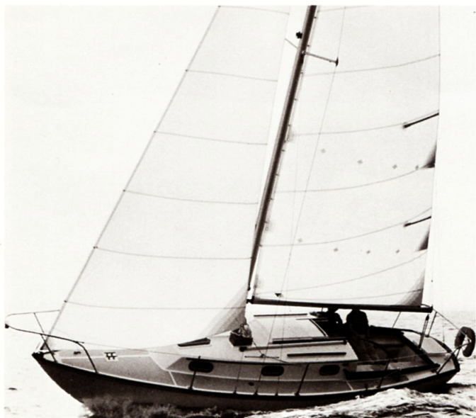
CAPE DORY 27 L.O.A. 27' 1" L.W.L. 20' 0" Beam 8' 6" Draft 4' 0" Displacement 7,500 lbs. Ballast 3,000 lbs. Sail Area 365 sq. ft. Designer Carl Alberg
