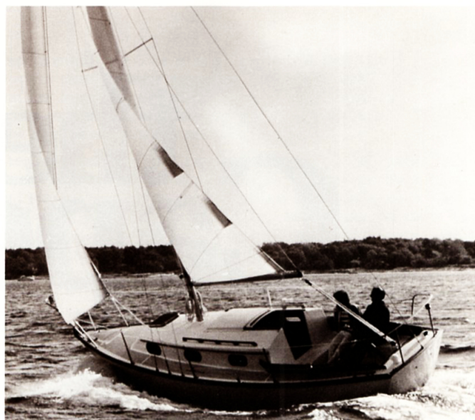
CAPE DORY 25D L.O.A. 25' 0" L.W.L. 19' 0" Beam 8' 0" Draft 3' 6" Displacement 5,120 lbs. Ballast 2,050 lbs. Sail Area 304 sq. ft. Designer Carl Alberg
