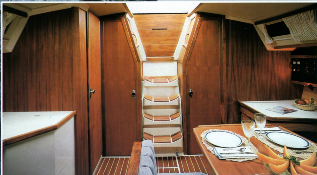
The main cabin: view aft. Note the angled ladder treads, the engine is fully accessible behind the hinged ladder unit. The teak doors outboard of the ladder are to the aft cabins. The head is to starboard, the navigation desk is to port.
