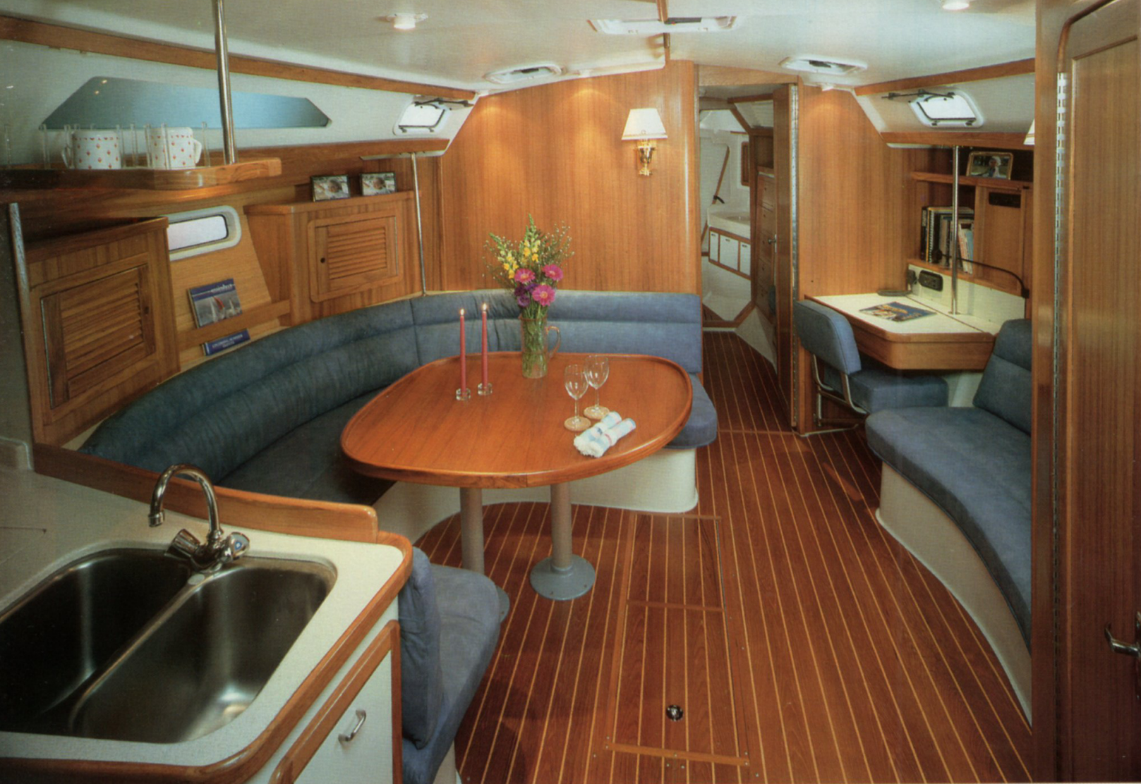
The two cabin interior features wrap-around seating frames the custom teak table, that lowers to form an additional berth. The larger navigation desk has enclosures for electronics and entertainment center. Large overhead hatches are complemented by adjustable task lighting throughout the main cabin.
