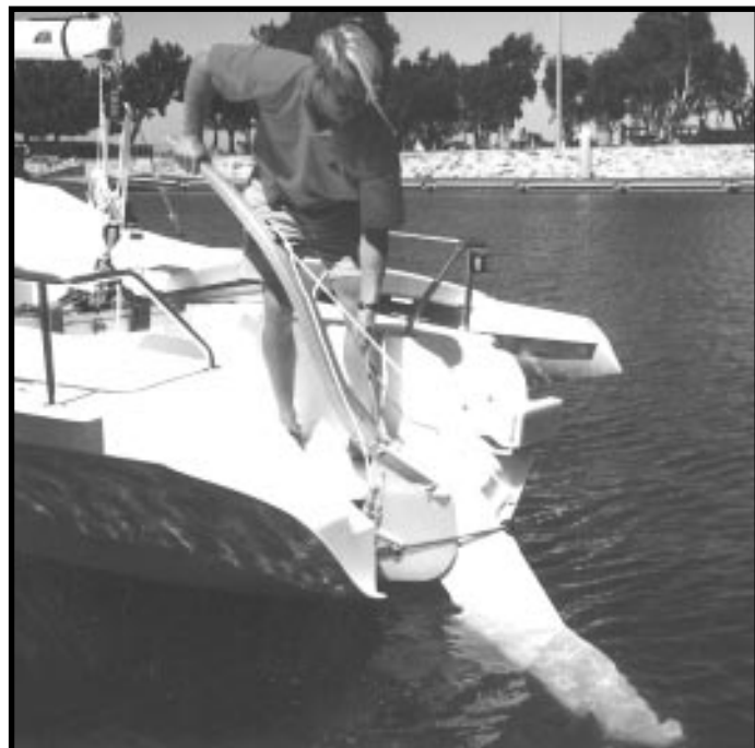
F-28 transom hung rudder being lifted up - note how tiller can give extra leverage by pull up line being cleated to it.
