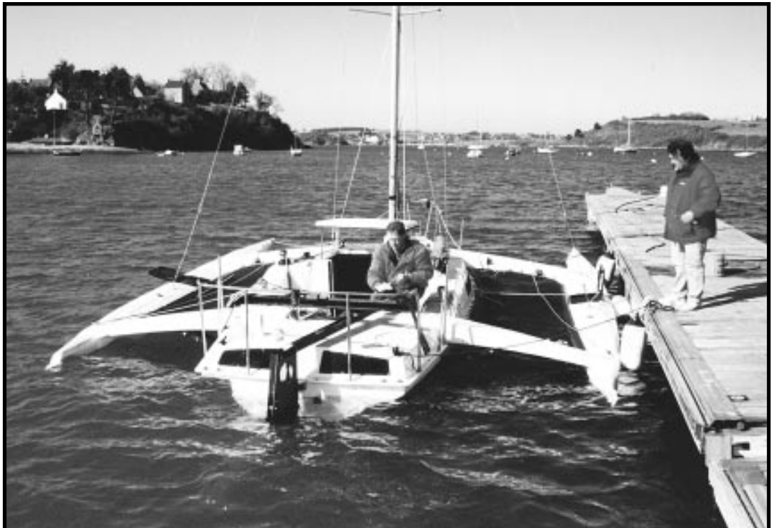
Even when fully flooded, a Corsair will stay afloat easily. This F-27 was deliberately flooded in order to demonstrate its unsinkability.
