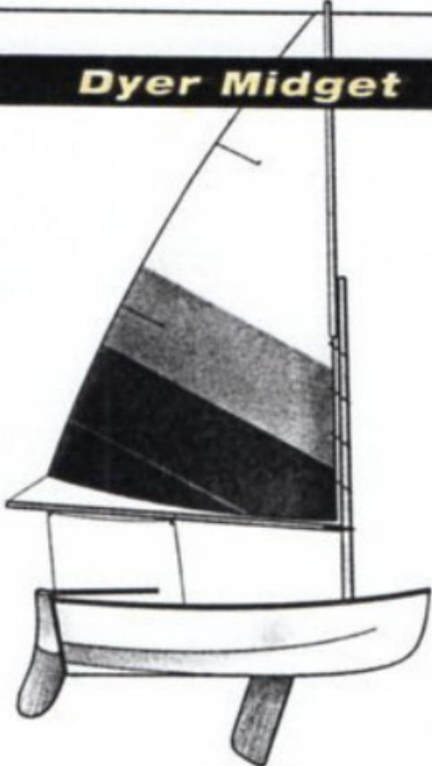
**This hard-chined fiberglass boat will carry three people or one person and a big pile of gear. The sailing version comes with a full daggerboard trunk. Sail, oars and oarlocks, rudder, and tiller are standard.**
