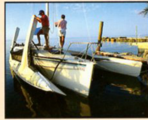
3. Single-handed folding or unfolding requires less than 3 minutes and the nets tension themselves automatically.
