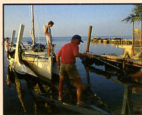
1. The mast is raised while on the trailer. Launching is with the floats still folded (you can even motor without lowering the floats, just like a powerboat).
