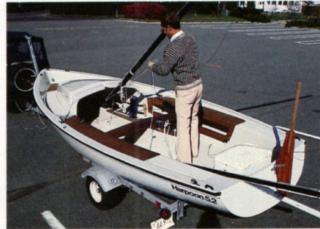
Raise mast with jib halyard. Mount boom and launch.
