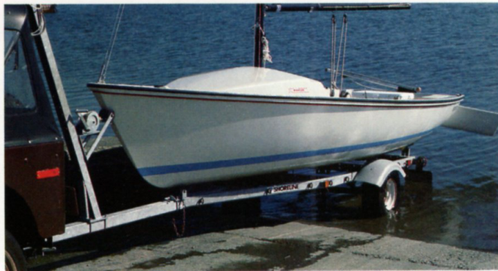
Unique, molded-in skag helps align boat on trailer.
