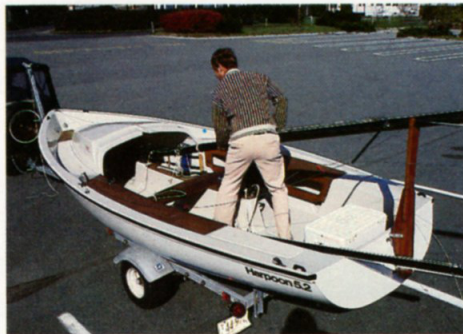
Slip the mast onto Harpoon 5.2's hinged step pin.
