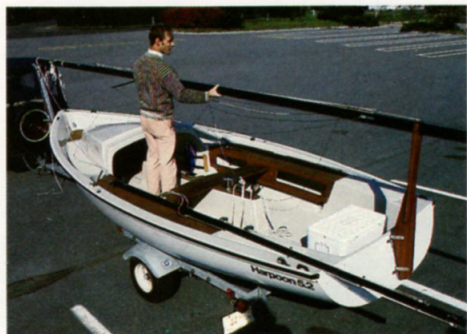
Mast rides securely on trailer and boom crutch.
