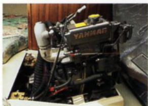
9 HP Yanmar diesel is standard, an 18 HP version is optional. Both afford great accessibility.
