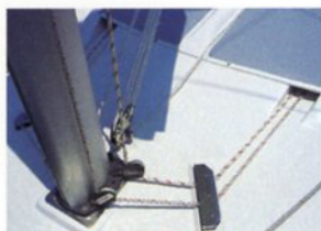
All lines lead aft for short-handed sailing.
