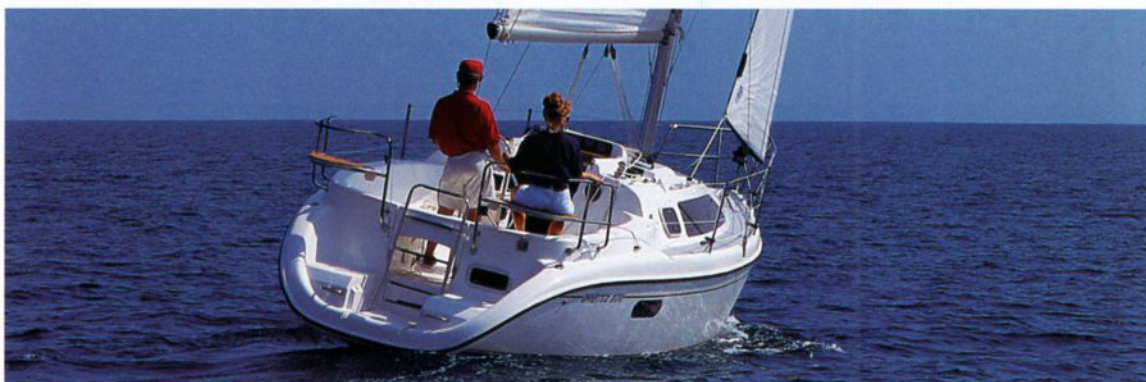
A walk-through transom, integrated swim platform, and stern rail with seats make the 280 transom really functional.
