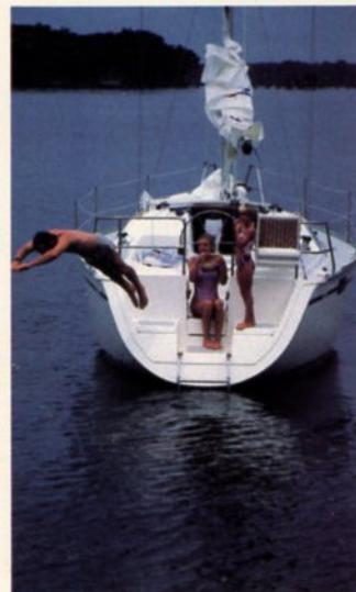
*Removing the arched helm seat opens the walk-through transom that includes steps and storage lockers. The ease of entry from the water is excellent for swimming, unloading the tender, as well as safety on retrieval. With the helm seat in place and the swim ladder raised, the deep cockpit returns to its full enclosure.*
