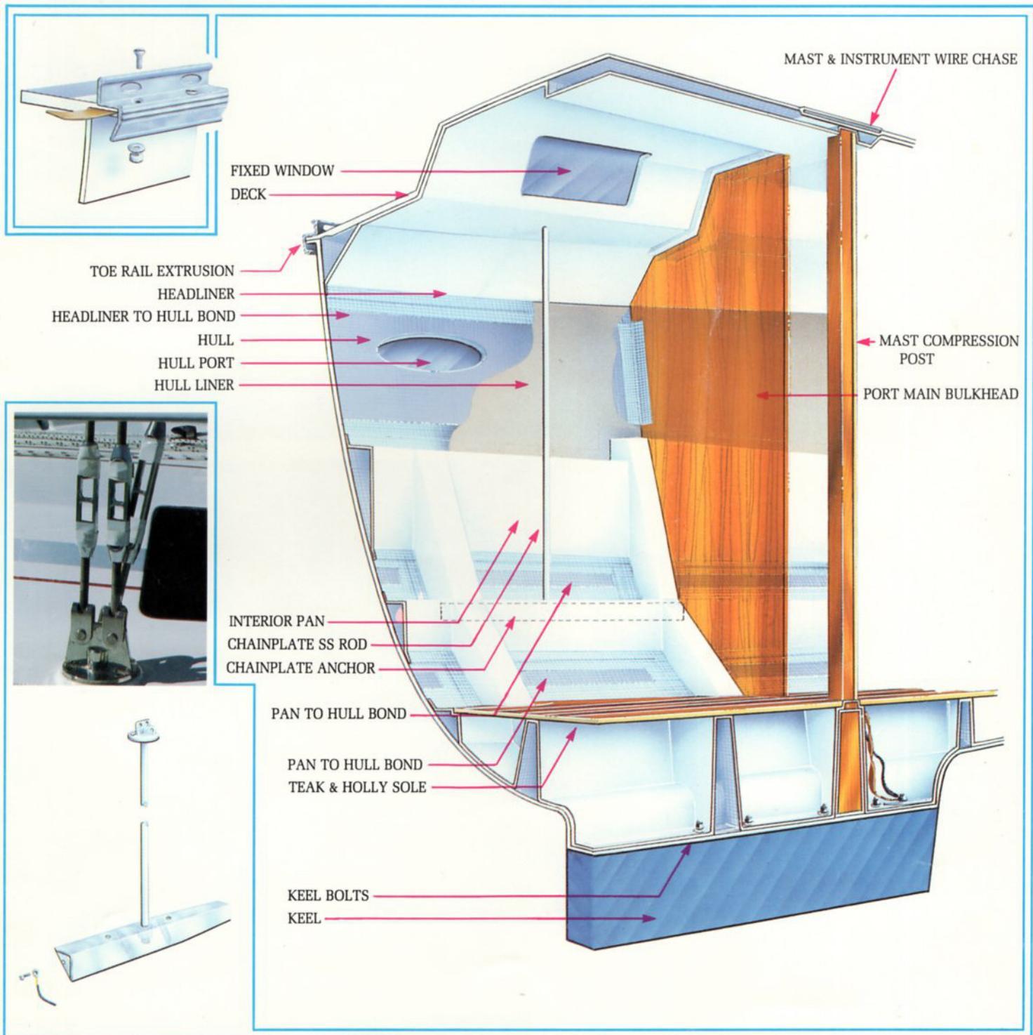
additional space below decks due to a single penetration of the chainplate through the deck to the frame.
