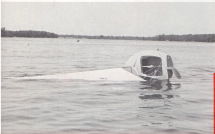
Safety is built-in with unique, unitized, non-swamping deck and cockpit, sealed mast and positive foam floatation.
