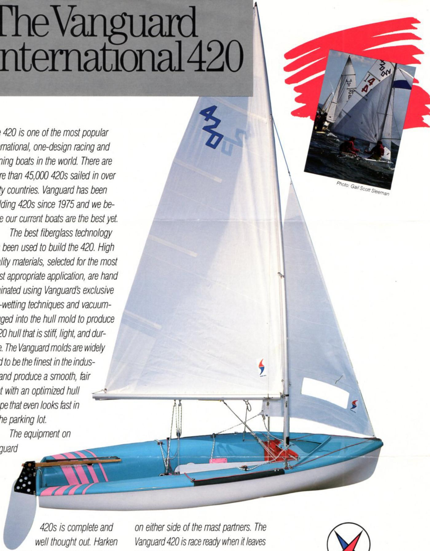
*420s is complete and well thought out. Harken blocks and cleats are standard and provide excellent sail control. Proctor spars are standard with either the Kappa or the C section available. Dual spinnaker bags matched to your deck color are mounted*
