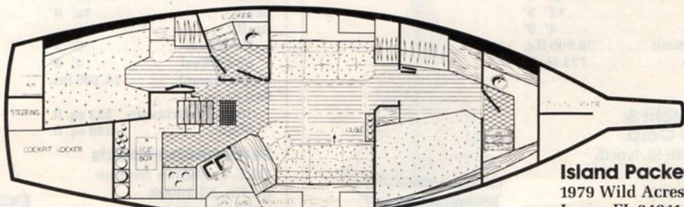
The integral hull and keel provide the strongest possible construction to withstand the stress of heavy seas and grounding. The moderate-draft full keel or optional shoal keel with centerboard give the capability for bluewater passages and cruising shallow coastal waters.
