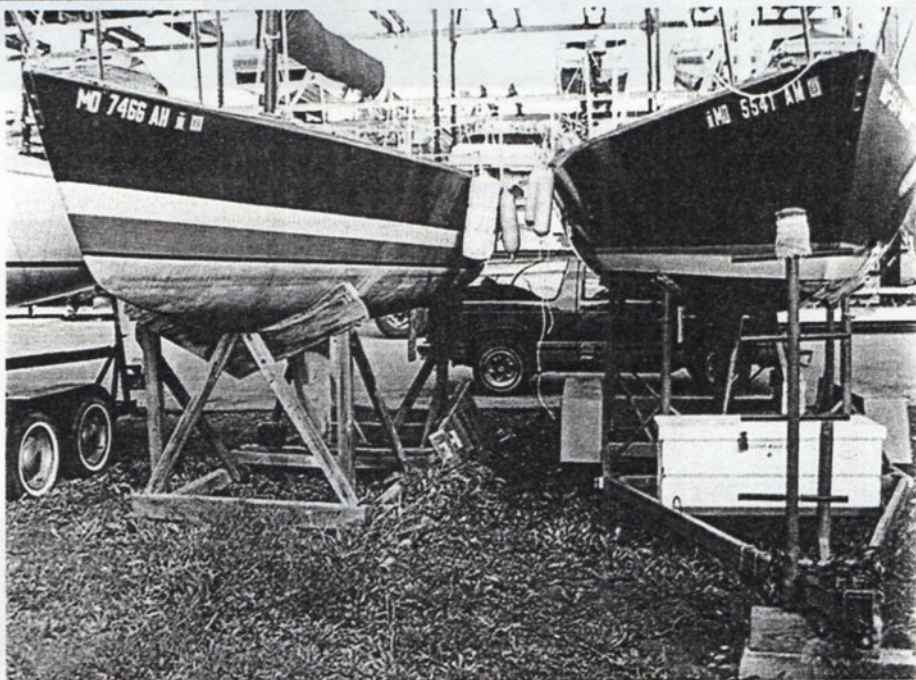
Right: You must decide how important a trailer is to you. In this yard, boats are launched with a huge fork lift. Here, a wooden cradle is great for a local racer, but just try to hit the road with that cradle.
