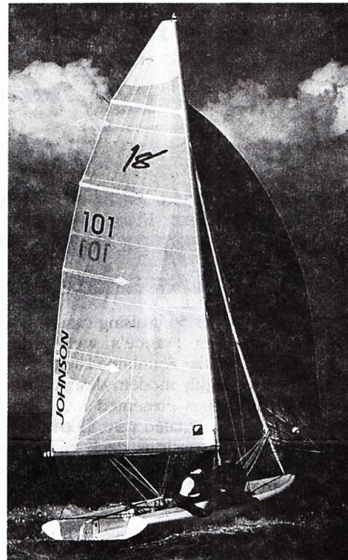
ated quickly on the new tack. Sailing on a broad reach with the 190-square-foot asymmetrical spinnaker up, it really took off, cutting cleanly through the waves. Setting the nylon chute is easy. The crew hauls two lines, one to move the carbon-fiber bowsprit forward about 2 1/2 feet, and the other to pull the tack of the sail out to the end of the sprit. As soon as the helmsman hauls on the halyard, the kite is up and flying. Acceleration is dramatic, but the boat remains stable and manageable.
