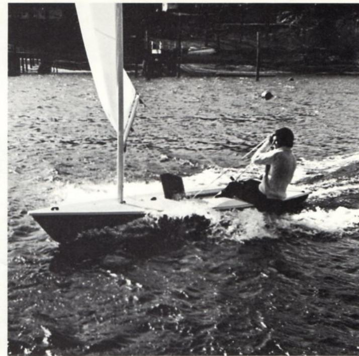
A carefully designed planing hull shape combined with light weight allows the Laser to jump up in a plane long before other boats of its size.
