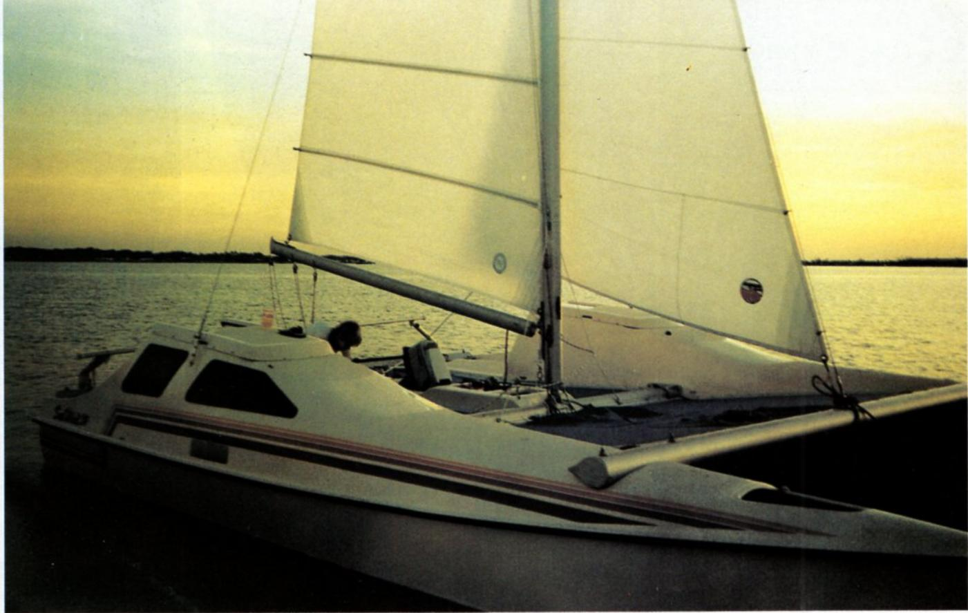
at the rudder castings or the cross beams will tell how the boat is built, but there are less obvious things too. Between the hand laid hull and floor there is positive foam flotation that will support almost one and a half times the weight of the boat. Even the trampoline track is our own extrusion so we can use a half inch bolt rope for maximum security.
