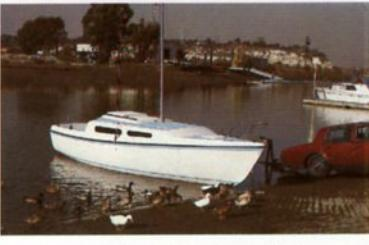
LAUNCHING: Back the trailer in until the boat starts to float free. Tie a line to the bow and give the boat a gentle shove. When the boat clears the trailer, pull it back to the ramp to pick up the crew. Reverse the process to return the boat to its trailer.
