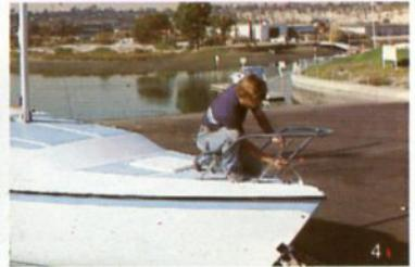
RAISING THE MAST: (1) Slide the mast to the rear and pin the bottom of the mast to the hinged mast step. (2) & (3) Raise the mast. It is light, and not too hard to lift. The load can be reduced to very little if a second person stands on the foredeck and pulls
