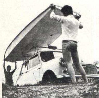
2. At 120lbs hull weight the MiniSail is simple for a man and a girl to get on or off the roof of a car and is light enough to be carried single handed down the beach.
