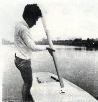
3. Join together the mast, slide it into the sleeve in the luff of the sail and rotate the sail round the mast. Slip the burgee into the pocket in the top of the sail. At the water's edge step the mast and unfurl the sail. Clip the clew to the boom and tie the tack line.
