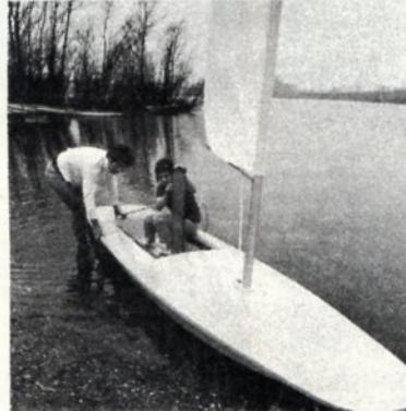
4. There are no shackles, no halliards, no wire rigging or bottle screws in the MiniSail. Once the sail is up just attach the mainsheet and kicking strap, instal the rudder and dagger board and your MiniSail is ready to sail.
