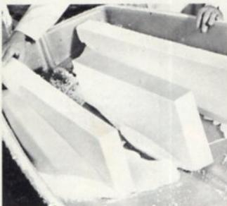
Foam blocks like these are bonded to the inner hull to make it virtually unsinkable.
