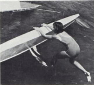
In event of a capsize, boat is usually easily righted by standing on board and pulling on edge of deck.
