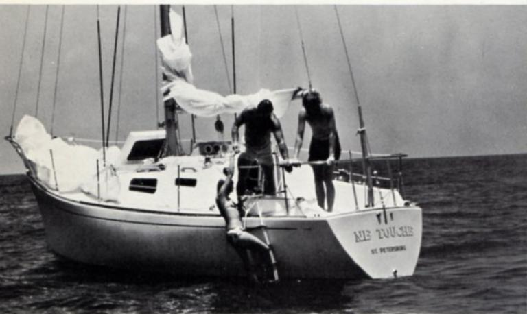
This 30-footer demonstrates how a contemporary racing yacht can be both fast and beautiful. With an overall length of 29' 11" she can top any MORC fleet. Then a long waterline, clean underbody, streamlined keel, light displacement and heavy ballast combined with a powerful high aspect ratio masthead rig are the primary reasons why the Morgan 30/2 has done so well in IOR competition.
