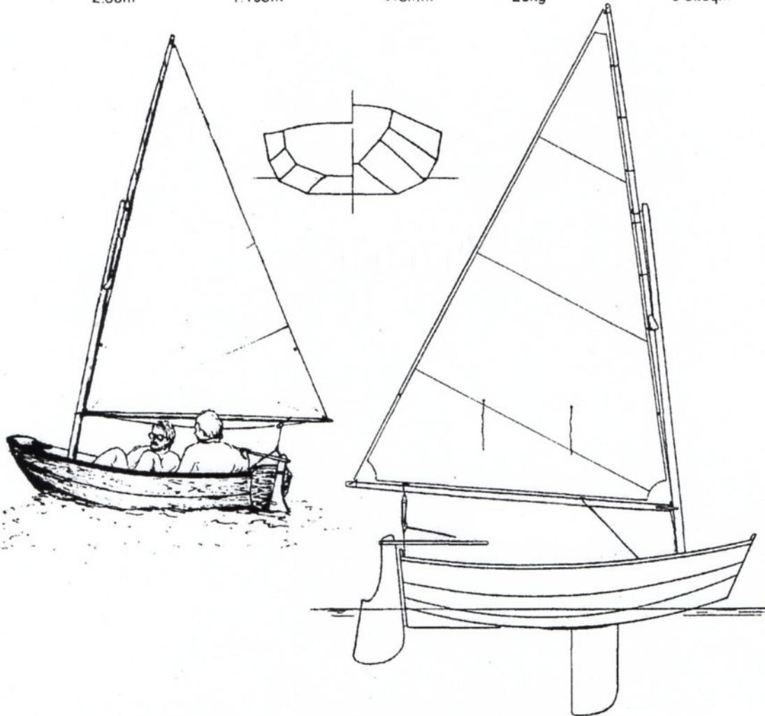
Type: flat-bottom pram, clinker sides   Optional rig: gunter with daggerboard or leeboard
