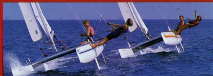
**DESIGN:** *Round Bottomed Symmetrical Hulls* - All NACRAs float on top of the water making them more maneuverable, dry and stable. Speed potential is greater because of a low wetted surface area.
