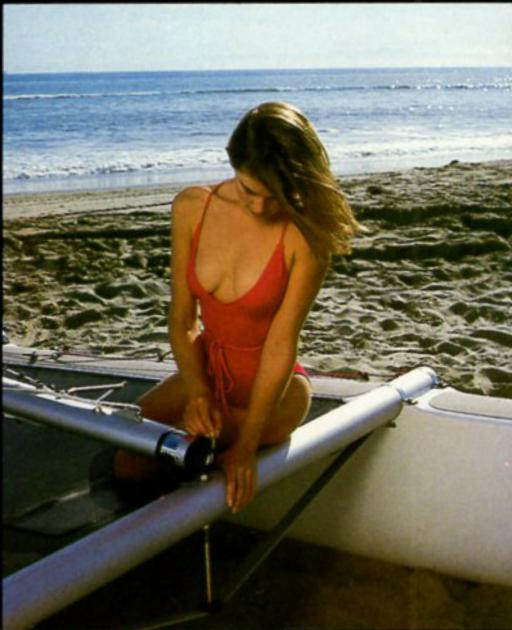
New ball and pin system makes stepping the mast faster and easier. Just put in place and drop on the pin.
