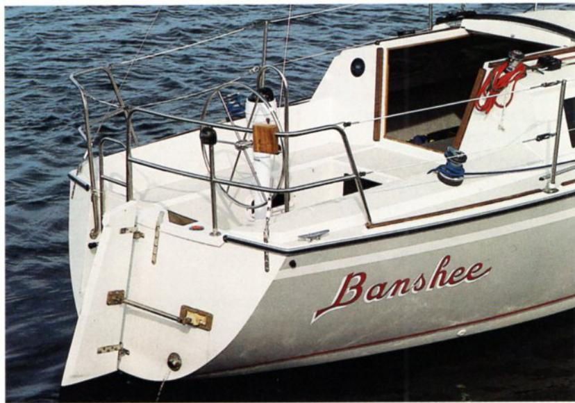
Readily apparent differences between the production O'Day 272 and the limited edition O'Day 272 LE are the LE's distinctive two-tone grey hull and deck, Edson pedestal wheel steering and inboard diesel engine.
