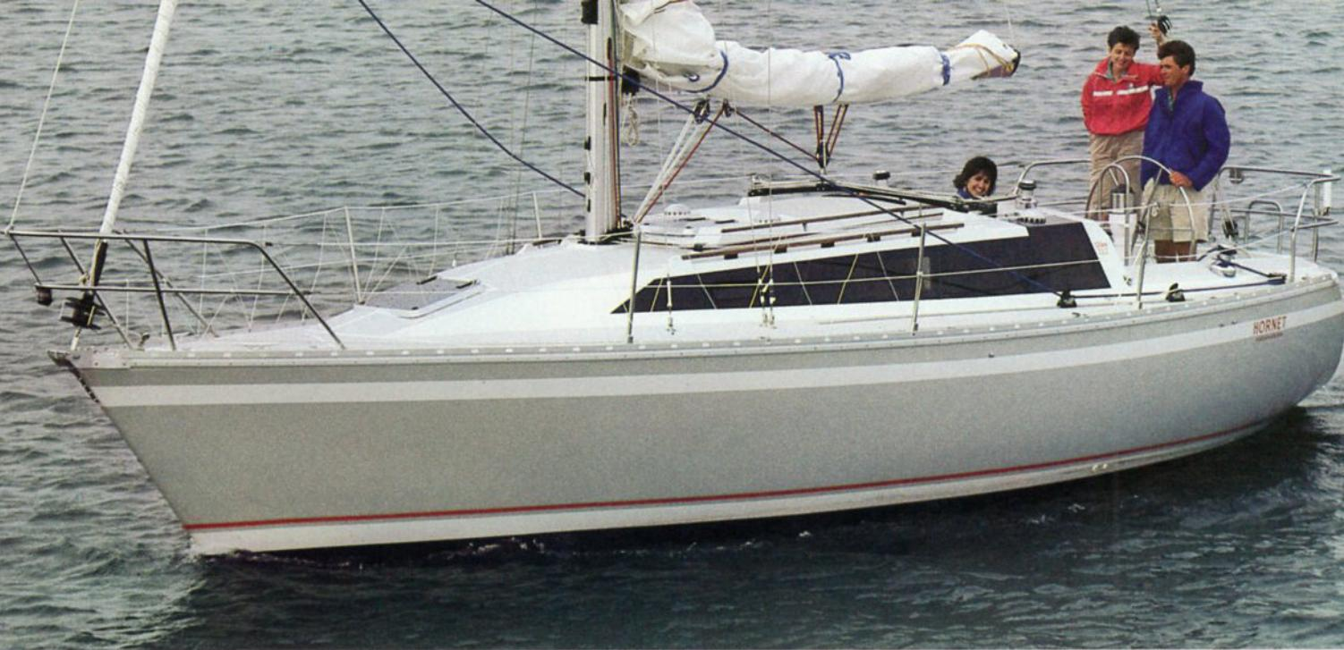
*Exterior handholds are firmly mounted teak rails and sturdy lifelines with stanchions bolted through the deck.*
