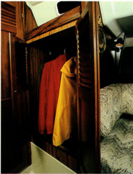
Use the hanging locker for foul weather clothing, it drains into the bilge.
