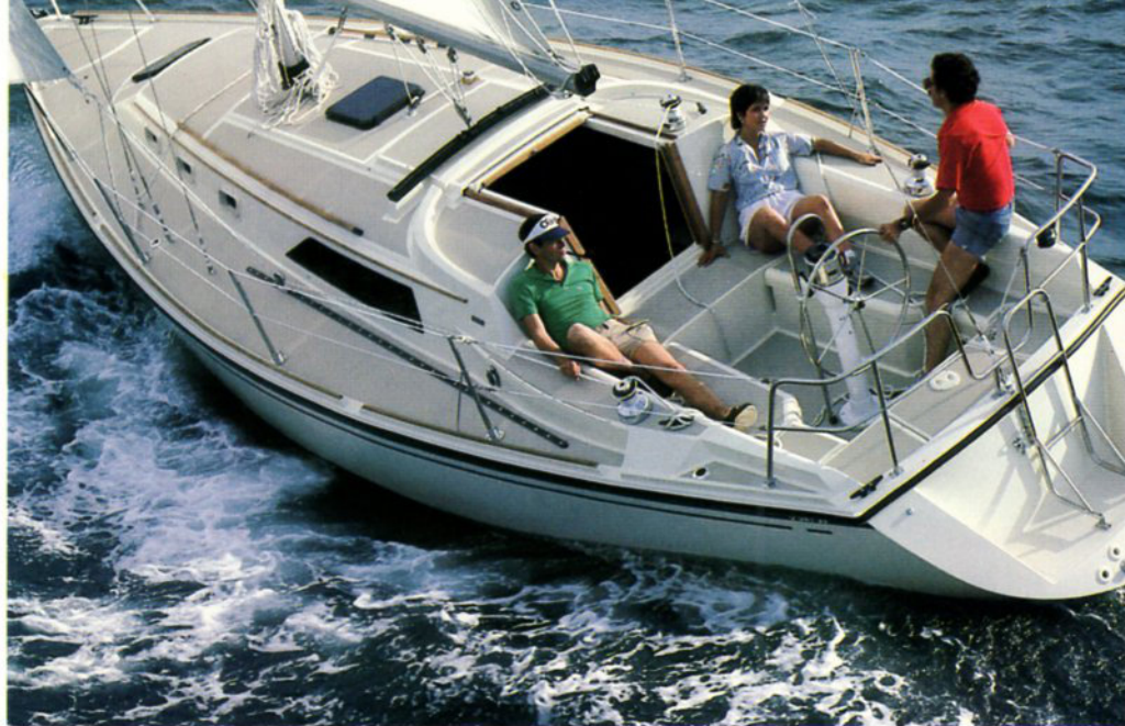
Cockpit is large, visibility over the house is unobstructed. Note the long genoa track for optimum sail trim.
