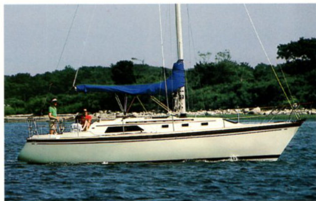
Attractive proportions of cockpit, house and fore-deck make the 35 a handsome vessel. Power is Universal diesel.
