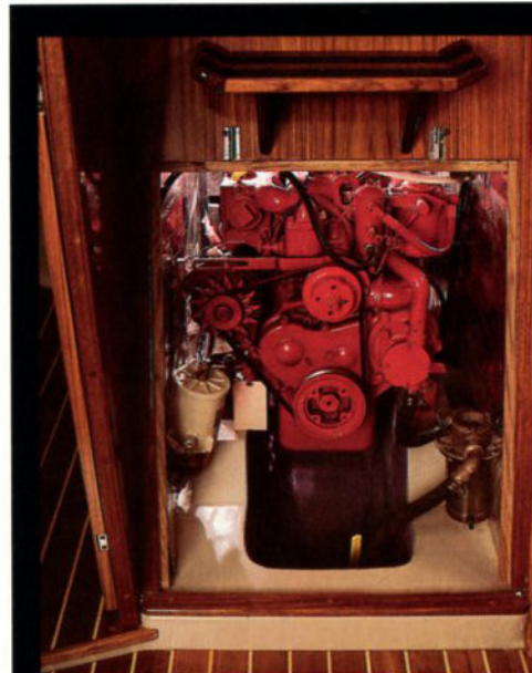
The FWC Diesel has excellent access from forward, above and in the filter-dipstick area.
