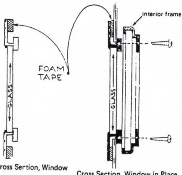
After a period of sailing, it is possible that some minor leaks may develop at the windows as they are designed to "float" on the foam tape strip. Any water which enters may be channeled between the hull and interior liner, finding its way aft to appear as a leak above the galley or quarterberths.
