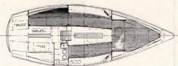
The cockpit is 7'3" long, with a fuel-tank storage bin to port, a large cockpit locker to starboard, and an anchor locker on the foredeck.
