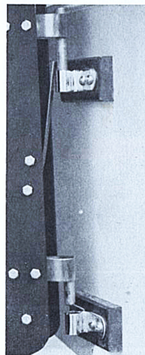
Mount the rudder head on the transom making sure the pintles are firmly located in the gudgeons.
