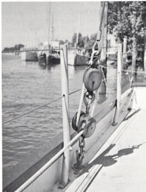
Wooden Cheek Blocks can be easily made by builder as can all staunchions, pulpit etc.,
