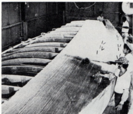
THE START OF A BALSA CORE DECK After the C-Flex is in place, it is wet down with resin
