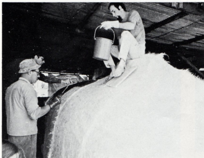
Here we see C.S.M. pre-measured and fitted to hull prior to application of resin.
