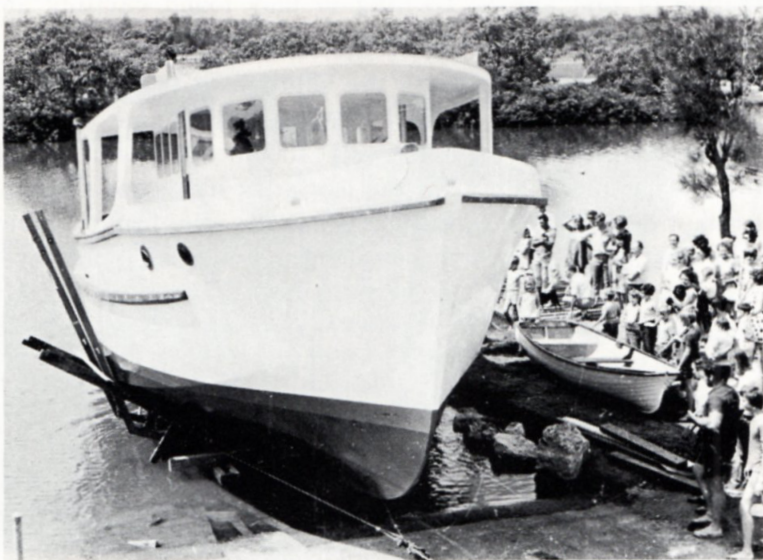
ROBERTS TRAWLER 45 female moulded in cheap ply mould at Marine Park.
