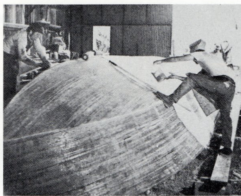
29 FT HIGH SPEED FISHING BOAT Additional laminations of fiberglass and resin are added over the C-Flex to build up the required hull thickness.
