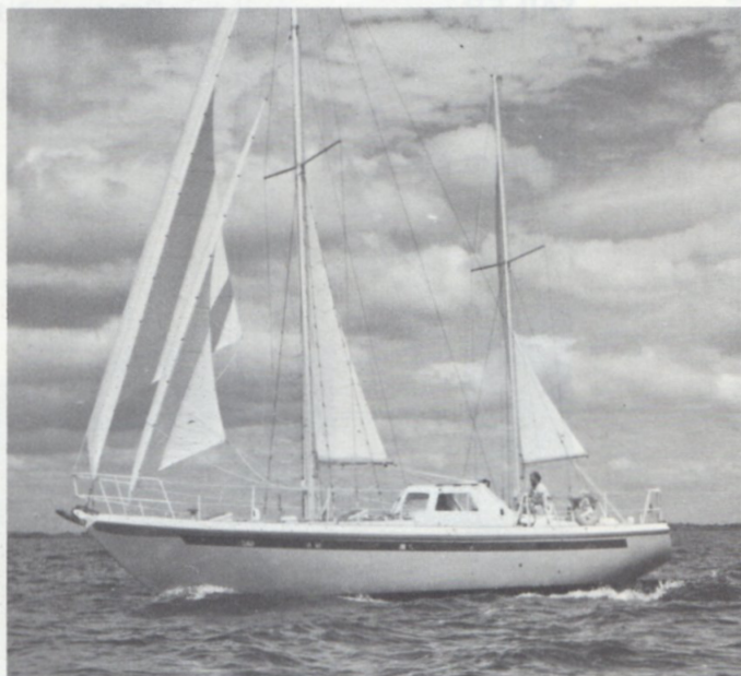
ROBERTS OFFSHORE 44 Fibreglass hull — plywood cabin — steel ballast — alloy fittings.
