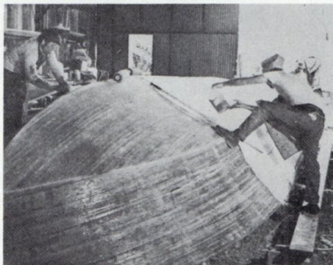
29 ft High speed fishing boat. Additional laminations of fibreglass and resin are added over the C-Flex to build up the required hull thickness.
