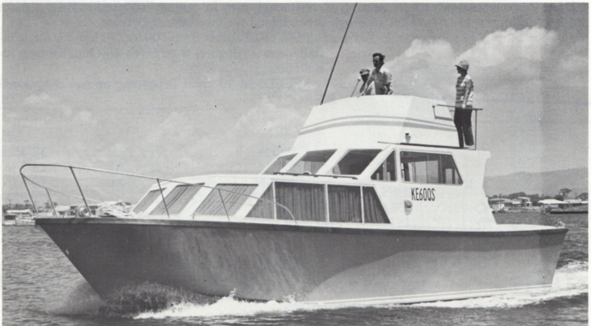
Amateur built Waverunner 36 — 20 Kts. with single 320 h.p. Cryslar.
