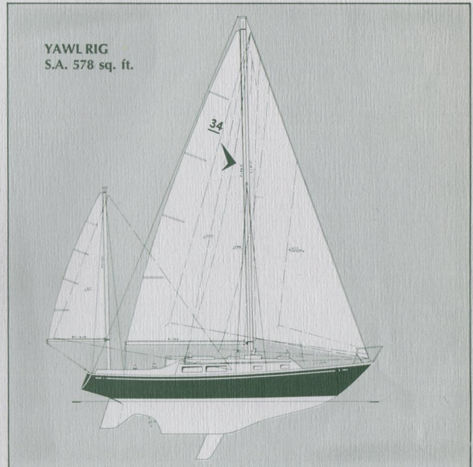
A high performance design from McCurdy & Rhodes. Aerfoil centerboard and aerfoil fin-and-rudder combination plus low wetted surface hull sections contribute to superior speed. "T" cockpit and SeaFlair™ spray rail will appeal to the racing man. Yet she is ideal for cruising with her truly spacious, comfortable interior and shoal draft. The Seafarer-34 is a yacht that will appeal to all members of the family and be a proud possession for years to come.
