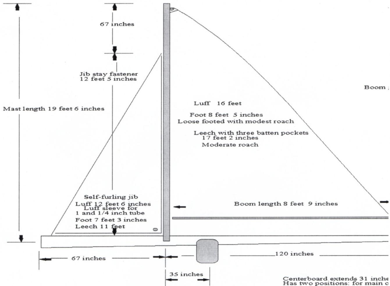
**Self furling jib roller** is 13 feet 5 inches bolt to bolt on 1 inch tube with 1 1/4 inch outer tube roll. Two shrouds (side stays) are fastened to the top bolt and secured to eyes on edges of deck, 16 inch Mast is jointed 10 feet up from bottom and sail groove (track) begins 48 inches from the bottom, 1
