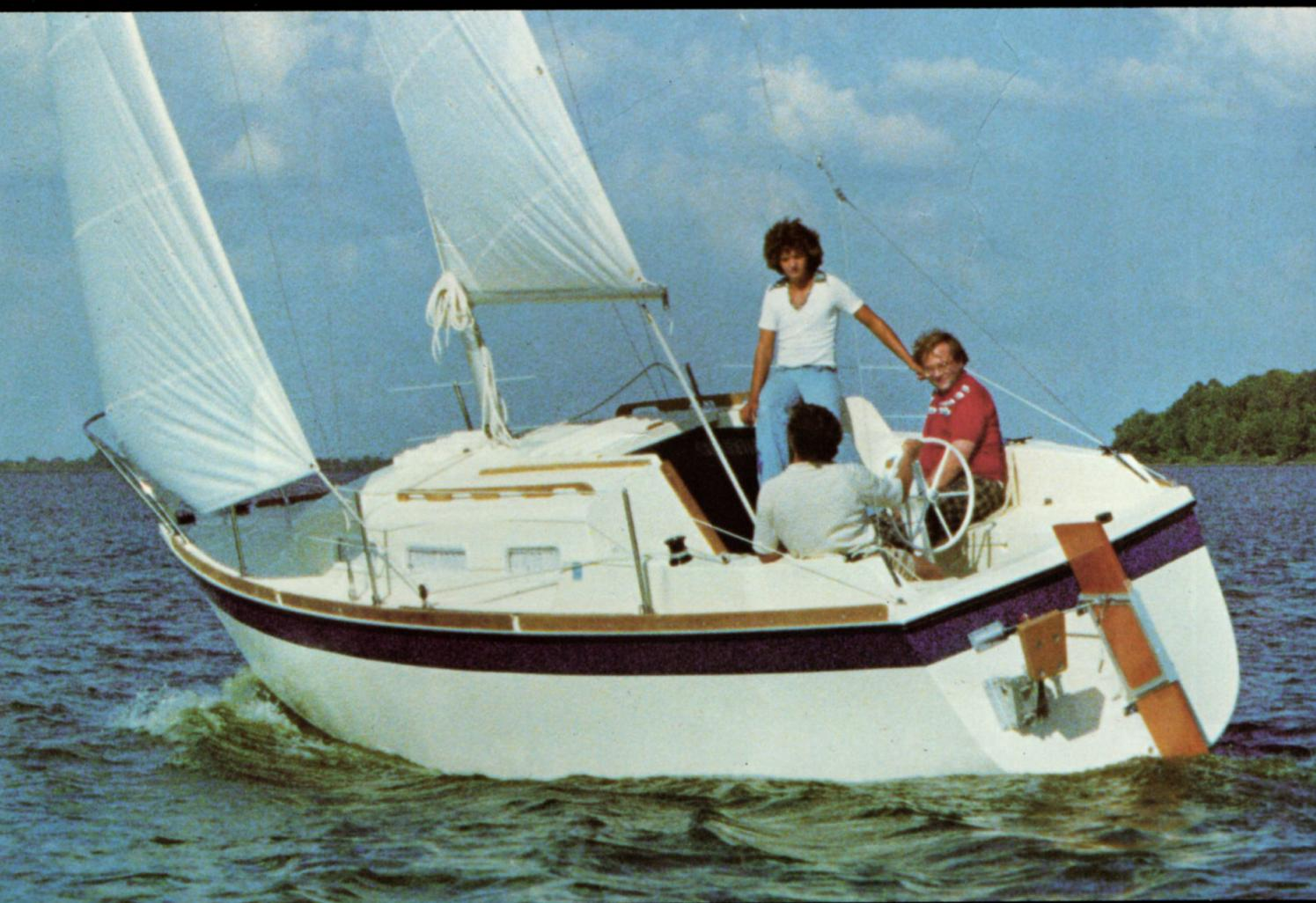
The roomy cockpit with its deep coamings comfortably accommodates everyone aboard. Some of the other outstanding features are a forward on-deck anchor locker, electric bilge pump, large smooth-finished sail lockers and out-of-the-way fuel tank storage. Gas or diesel inboard power is optional.
