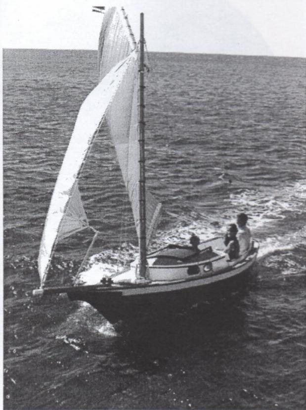
With a simplified construction, the project was turning out to be very inexpensive—as well as ultra-light (475 lbs, ready to finish and rig). This meant easy trailering and launching, and quick-handling performance under sail.
