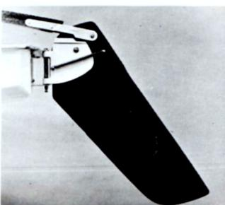
Smooth-working kick up rudder with spring action automatically lifts blade when beaching.
