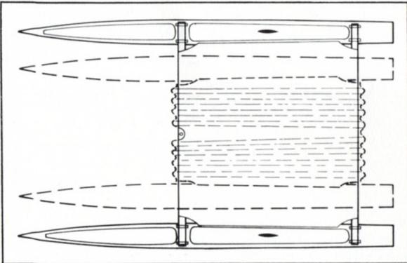
Telescoping crossbeams - you can take your 12 foot wide Super Cat on a normal 8 foot wide car trailer using our telescoping crossbeams. Set-up time is super quick. Pull the crossbeams apart to 12 feet then raise the mast, and you're ready to sail.
