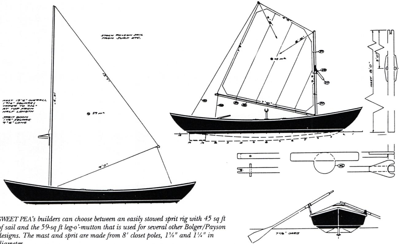
*SWEET PEA's* builders can choose between an easily stowed sprit rig with 45 sq ft of sail and the 59-sq ft leg-o'-mutton that is used for several other Bolger/Payson designs. The mast and sprit are made from 8' closet poles, 1½" and 1¼" in diameter.
