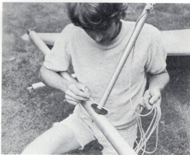
Attach the front stay using 5/8 in. clevis pin and key.
