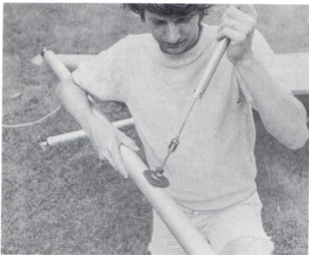
Attach the front stay using 5/8 in. clevis pin and key.
