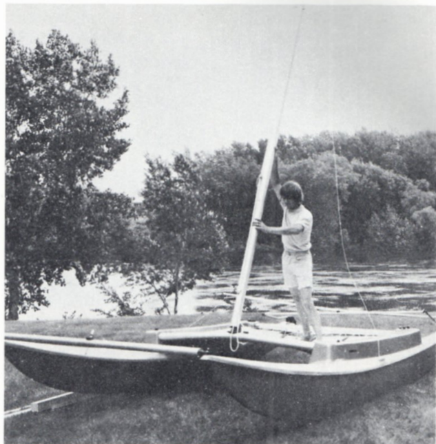
Slide the prewound jib sail and jib pole over the front stay.
