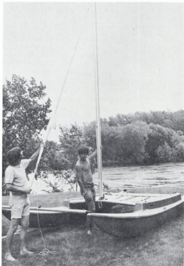
Slide the prewound jib sail and jib pole over the front stay.
